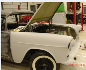
The '55 Chevrolet starts 2006 with all its body work completed and in primer.
