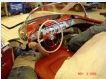
Jack & Chuck up-ended in '54 Corvette for windshield installation.
