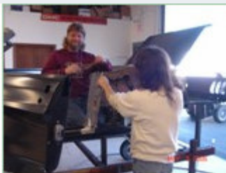
Ed & Jack fit the rear quarter on the '68 Mustang.
